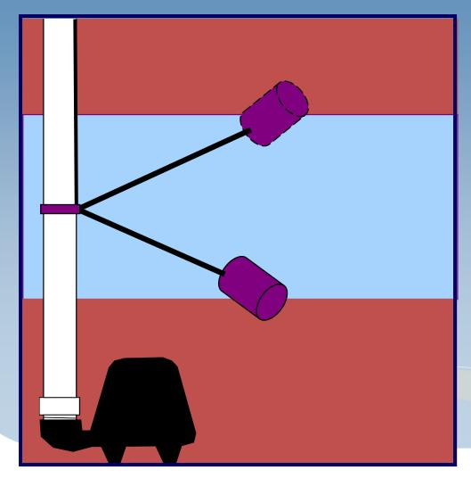
The best location for a switch is for the pump to always be submerged in a septic application!
