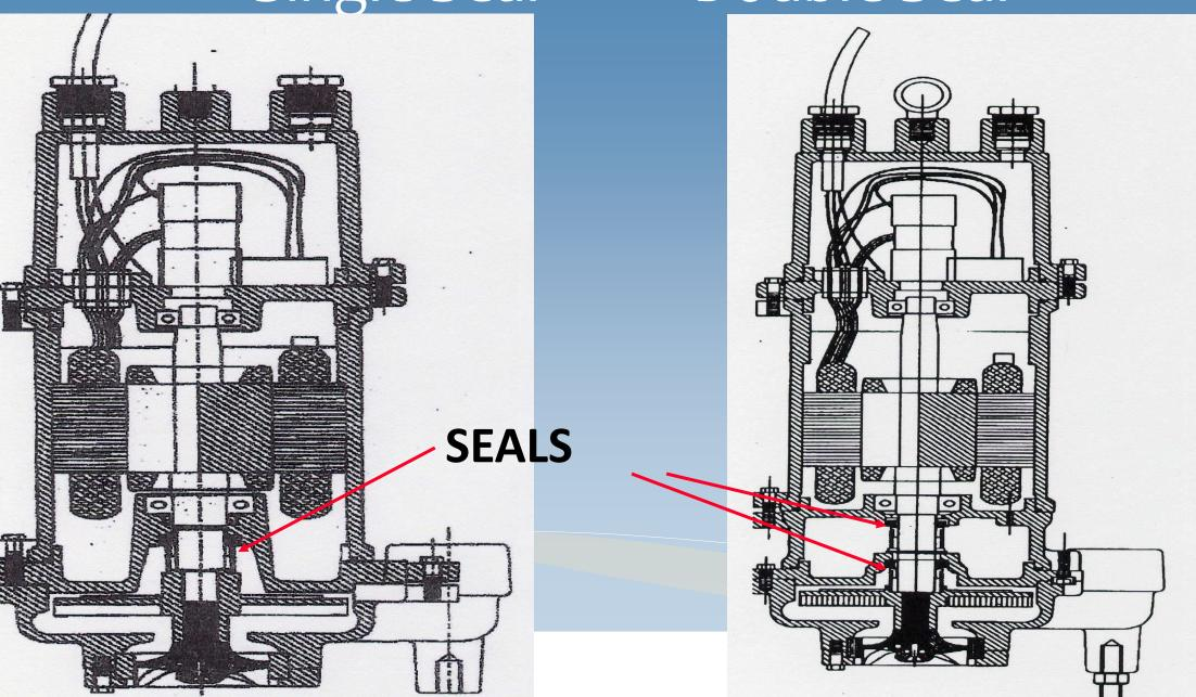
• What is the difference between a Grinder Pump and a Sewage Ejector?
