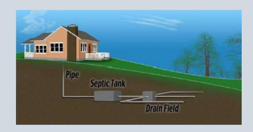
All wastewater is collected in the septic tank. There is generally a separation wall or settling tank for solids.
