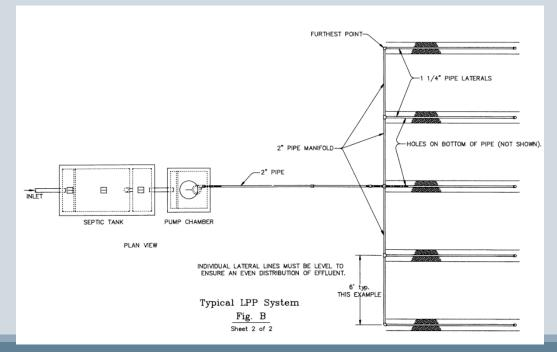
\*The operating head, also known as "squirt height" is the pressure required at each lateral hole to properly maintain the system. This head is added to the total dynamic head.
